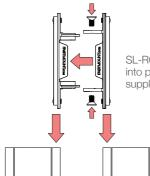
SL-RCAB180 and SL-RCF90 slide into profile groove and fastens with supplied grub screws.
